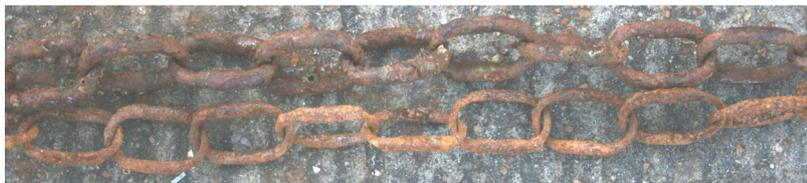
One length of chain within the same system can corrode quicker in some places than others.
